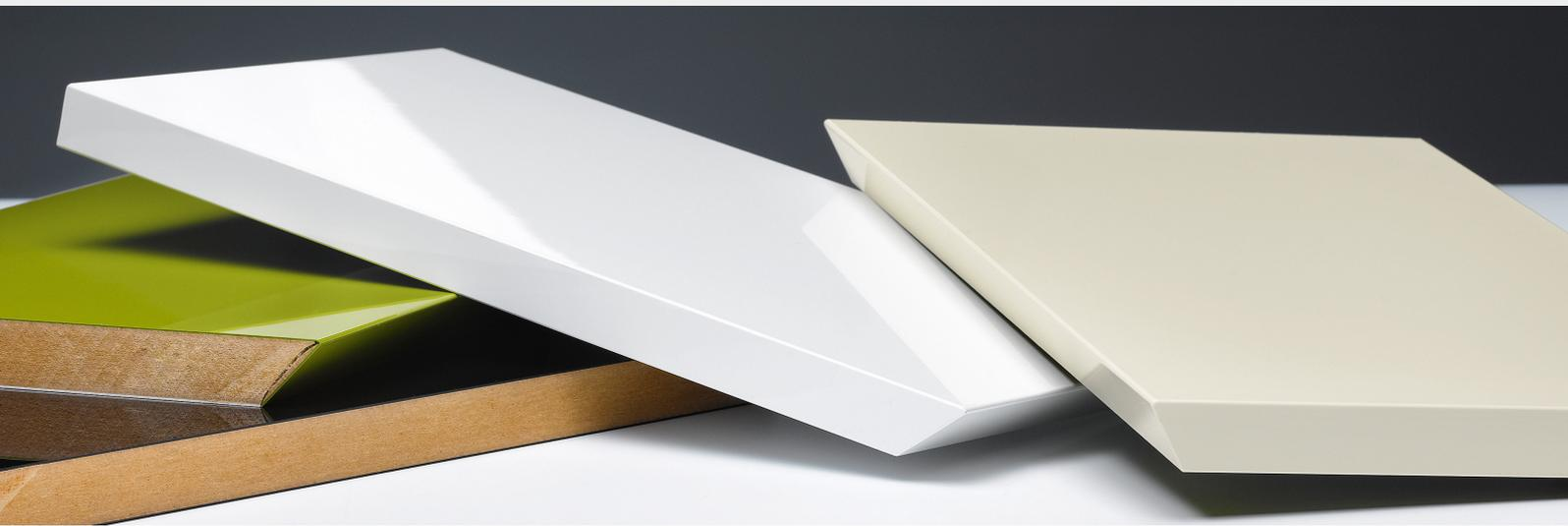
Preforming is a specific method of edge processing, in which the surface material is formed and curved around the edge instead of just gluing an edge on the panel. This method can be used on two opposite edges of a part of the furniture and provides the advantage of a non-visible joint between the surface and the edge.
